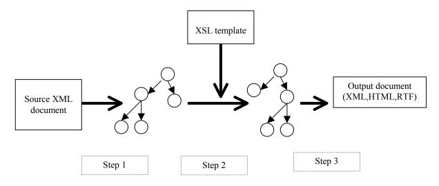
The process includes the following steps: the source document (XML) is translated into some tree representation (step 1), then according to the rules in the XSLT stylesheet the original tree is transformed into a new tree (step 2) and finally the result is serialized to file (XML. HTML, WML, etc.)
