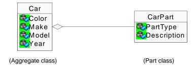
The class at the Car end of the aggregation relationship is sometimes called the Aggregate class (represented by a diamond at the end of the connecting line). The class at the CarPart end of the aggregation relationship is the Part class, instances of which are contained or
